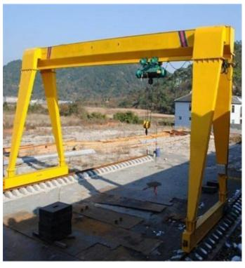
About the main beam and support leg, there are two types: box type and truss type, box type is good techniques and easy fabrication, truss type is light in dead weight and strong in wind resistance. The complete machine features light dead weight, simple structure and easy installation and maintenance and widely used.
